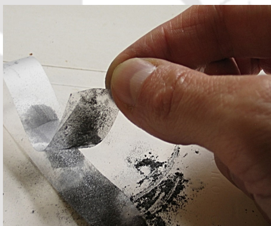
FIGURE 1.15: Schematic of scotch tape method to prepare graphene 5 .
