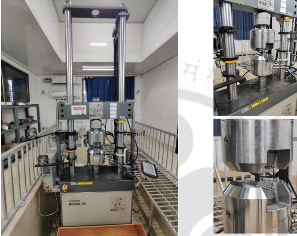
Fig. 4.6. 250 KN Servo Hydraulic Universal Testing Machine (Make: BISS, Model: MEDIAN 250) with pressboard sample
