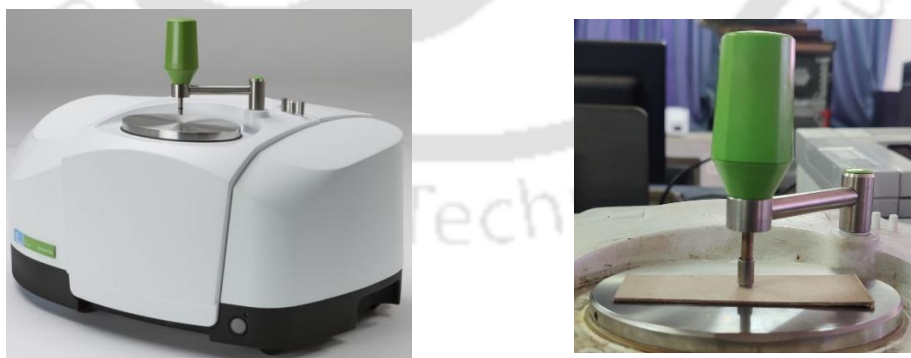
Fig. 4.5. FTIR Spectrophotometer (Make: PerkinElmer, Model: Spectrum Two)
