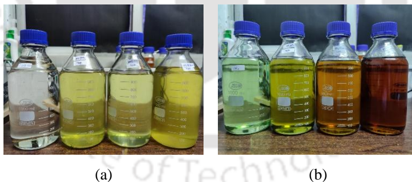
Fig. 2.4. a) Thermally Aged MO Samples at 0, 90, 200, and 500 hours b) Thermally Aged FR3 Samples at 0, 90, 200, and 500 hours.
