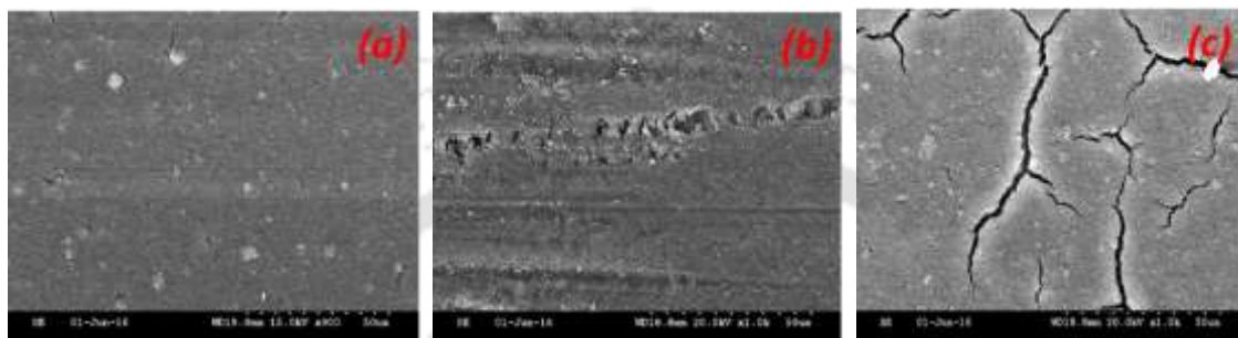
Figure 3.1 The SEM images of various thickness \text{TiO}_2 photoanode (a) 9 \mu\text{m} , (b) 12 \mu\text{m} and (c) 14 \mu\text{m} .
