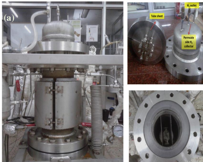
SS 310 MEMBRANE REACTOR (left), Reactor Bonnet & Tube Sheet (right up) and Reactor Shell with Baffles (right bottom)
