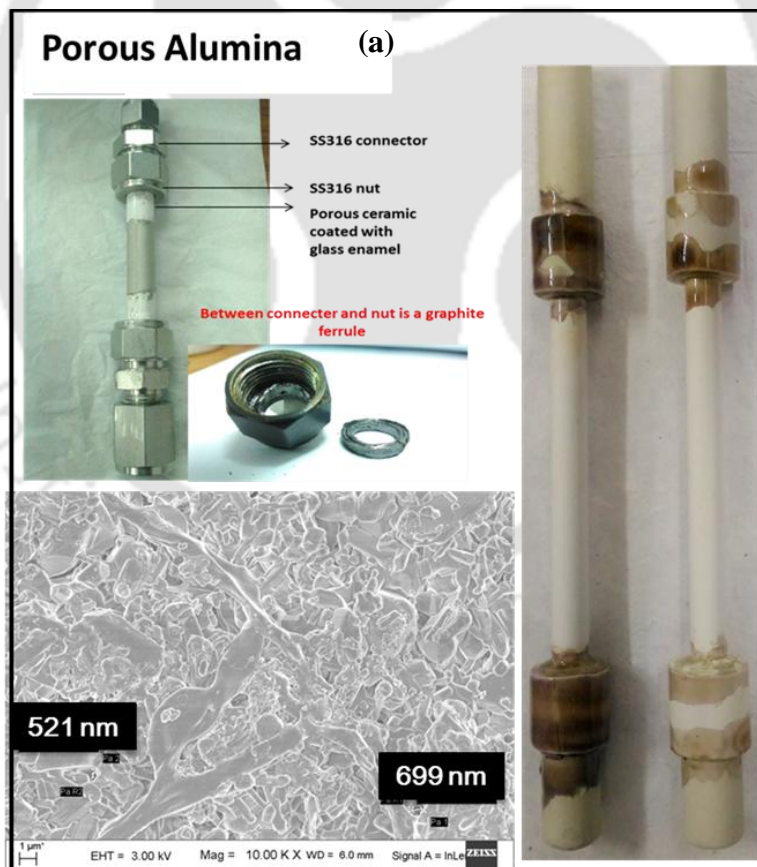
Fig. 2.4a Support assembly FESEM images of porous alumina
