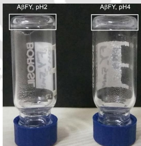
Figure 3.2 Gelation caused by 5 mM AβFY at pH 2 and 4 as assessed by inverting the tube. The gel area is marked with white rectangles.
