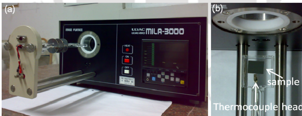
Figure 2.4: (a) Photograph of the table top RTA setup, and (b) magnified view of the sample holder.
