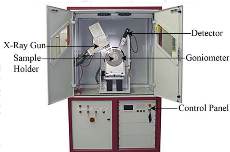
Figure 2.8: Photograph of the x-ray diffractometer (Seifert 3003 T/T, GE, USA) used for the structural characterization of the NWs.
