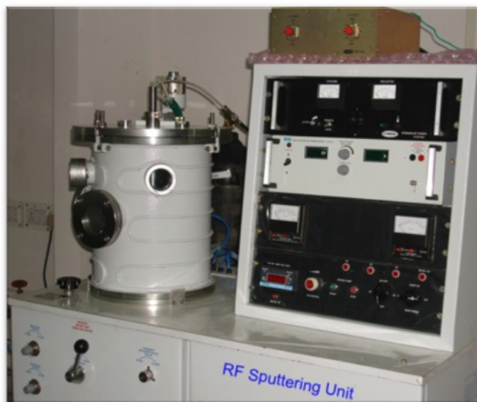
Figure 2.3: Photograph of the magnetron sputtering system (Hindhivac, India) used for the preparation of high quality ZnO seed layer.
