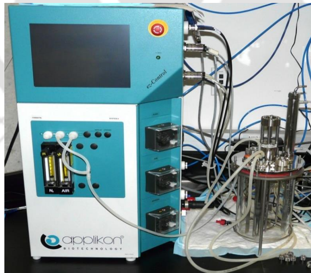
Fig. 3.1 (a) Schematic and (b) image of the stirred tank fermenter with control for fungal chitosan production for paper mill wastewater using P. citrinum .
