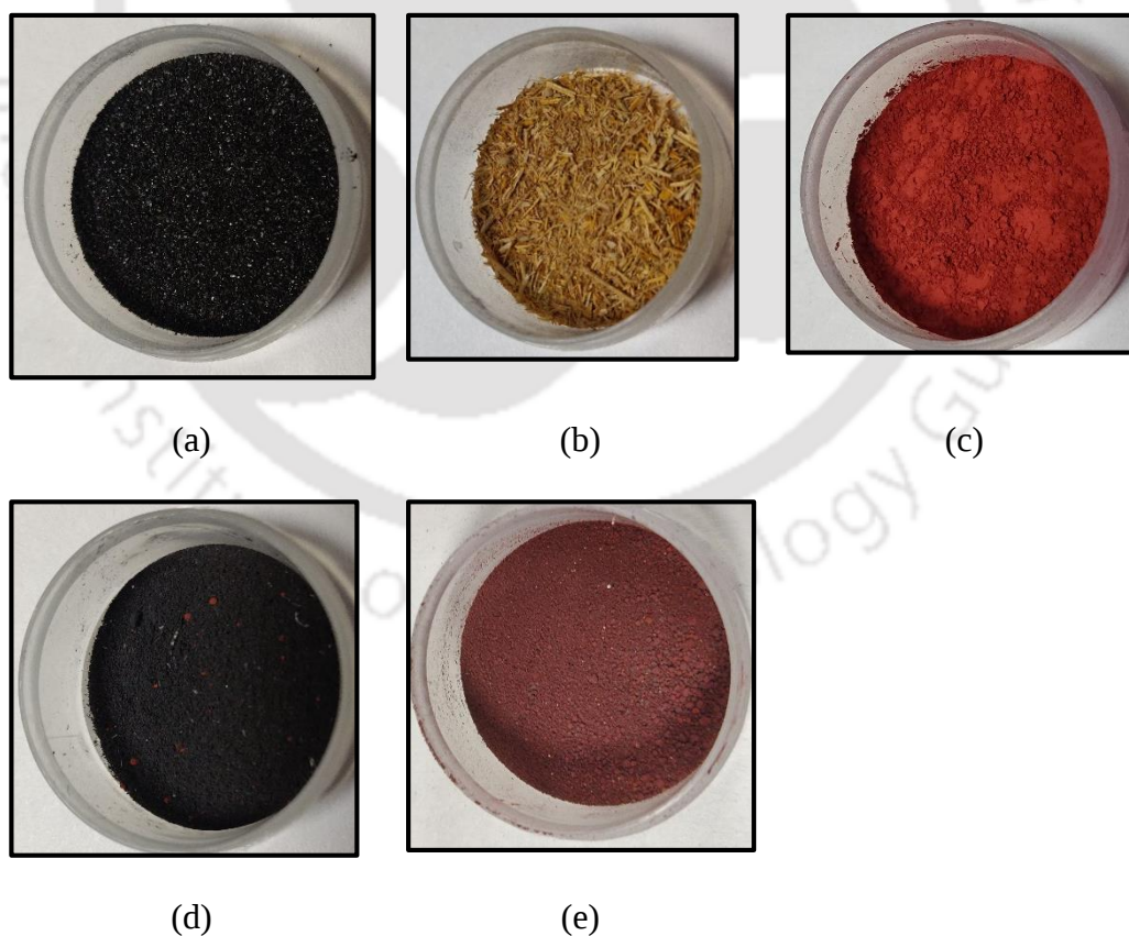
Figure 4.10. Photographs of (a) fresh LAC, (b) fresh RS, (c) fresh \text{Fe}_2\text{O}_3 , (d) reduced form of \text{Fe}_2\text{O}_3 obtained during CLC (e) re-oxidized \text{Fe}_2\text{O}_3 obtained from air reactor.
