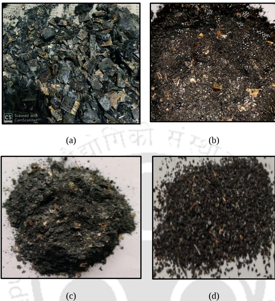
Figure 5.6. Snapshot of residue retrieved after (a) pyrolysis, (b) gasification, (c) combustion, and (d) screening of OPCB after combustion.
