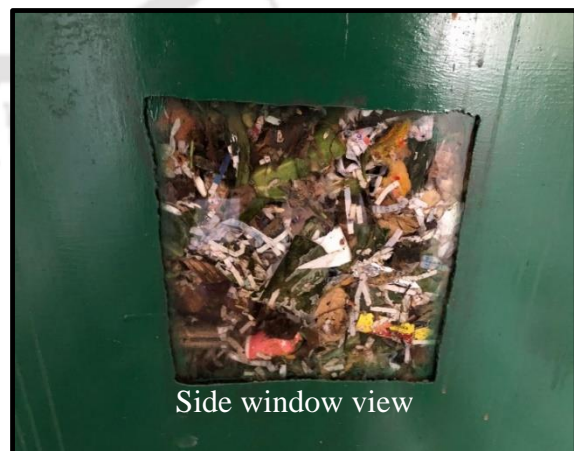
Fig. 4.7. Pictorial view of landfill simulation reactor
