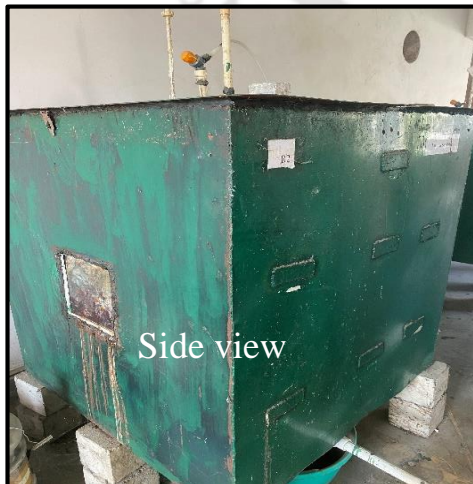
Fig. 4.7. Pictorial view of landfill simulation reactor
