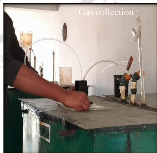
Fig. 4.9. Pictorial view of the collection of landfill leachate and gas samples
