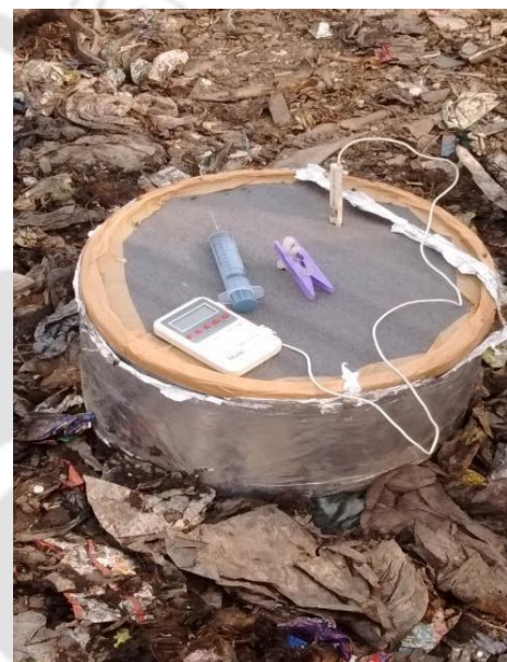
Fig. 4.5. Field setup of stainless steel chamber for gas collection
