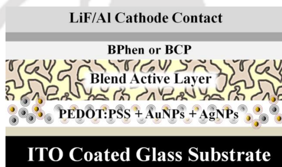
Figure 5.4. Schematic of the fabricated plasmonic bulk hetero junction solar cell.
