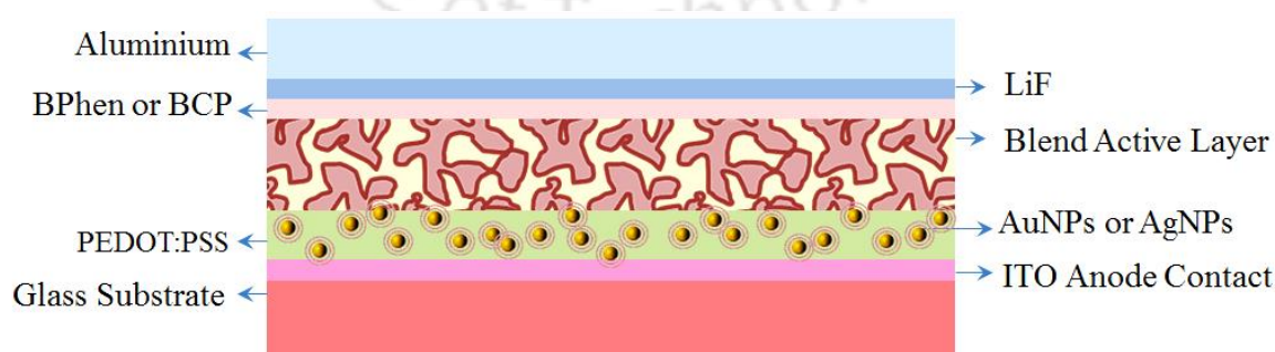
Figure 4.1. Schematic representation of the fabricated rrP3HT:PC 61 BM and rrP3HT:PC 71 BM based plasmonic BHJ organic solar cell.
