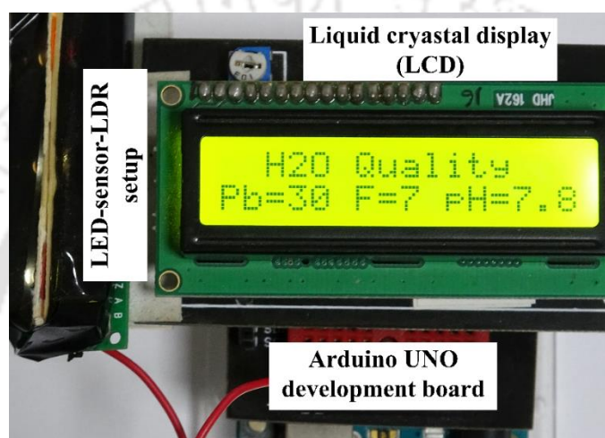
Figure 5.4: Image shows a POCT device for monitoring of F^- , Pb^{2+} and pH of water.
