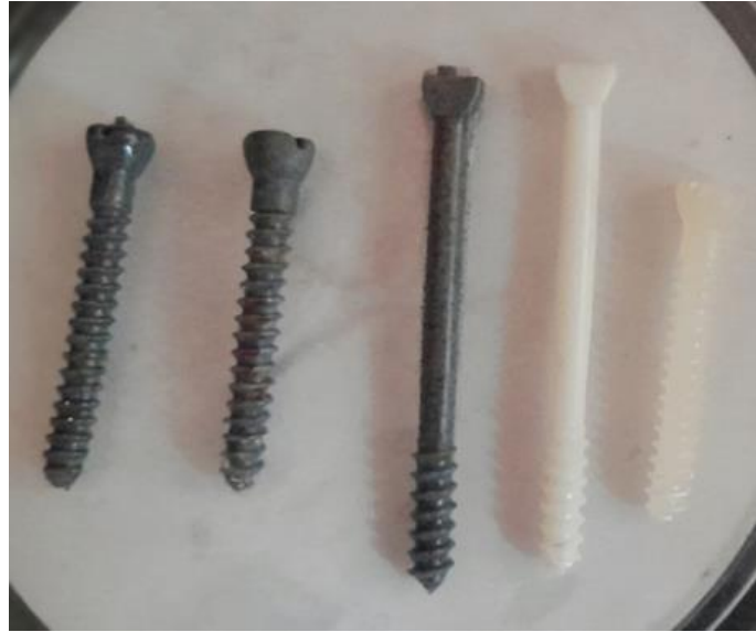
Fig. 6.2: Fabricated screw from PLA-based bio-composite as per ASTM standards by extrusion cum injection molding.
