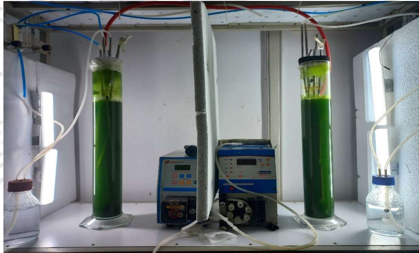
Fig. 6.11. Photobioreactor setup with a high culture cell density of 3.23 \pm 0.23 , using a 2-liter working volume. This was achieved by applying an optimized calcium-induced fed-batch process with CO 2 modulation over a 23-day cultivation period. Results represent the mean of n = 2 biological replicates; error bars indicate the standard deviation of the replicates.
