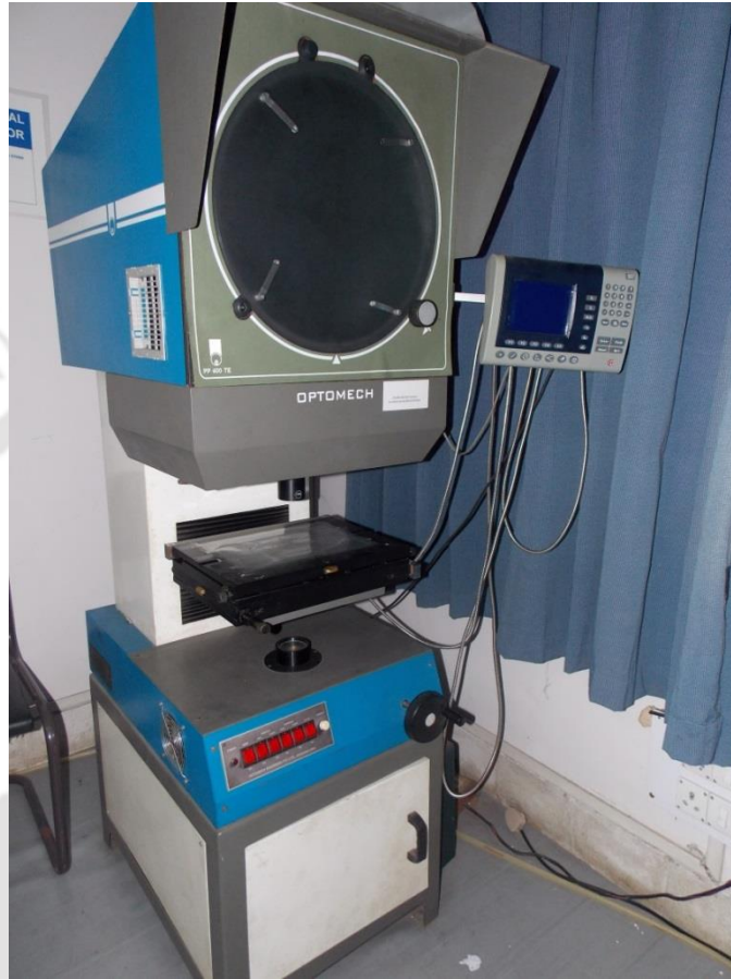
Figure 3.2 Optical profile projector (Model: PP400 TE, make: Optomech)
