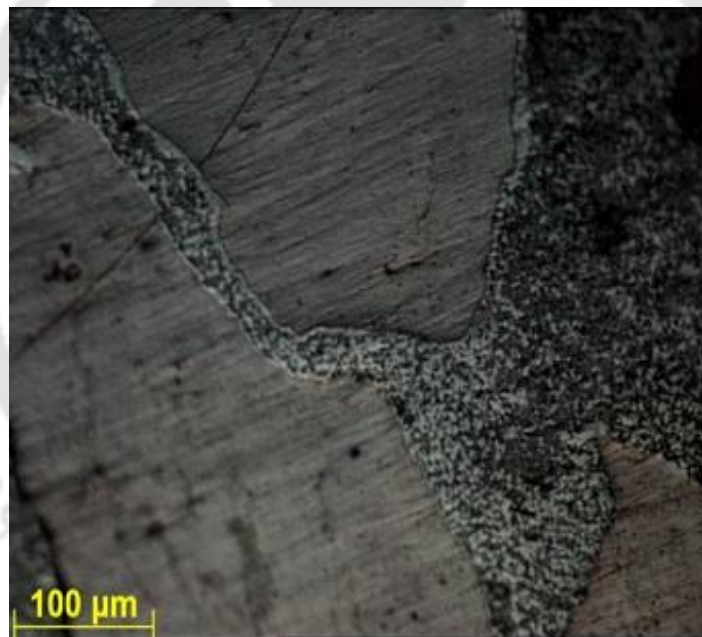
Figure 7.15: The Cu chunks move towards the Al side is visible here.
