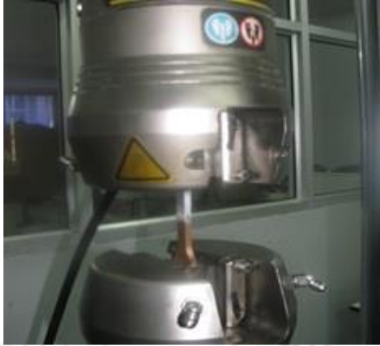
Figure 7.13: Instron-8801 tensile testing machine with AA6061- Cu B370 weld sample.
