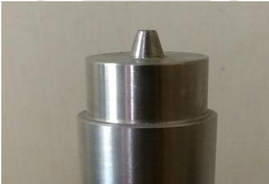
Figure 3.17: Conical pin geometry used to perform welding.
