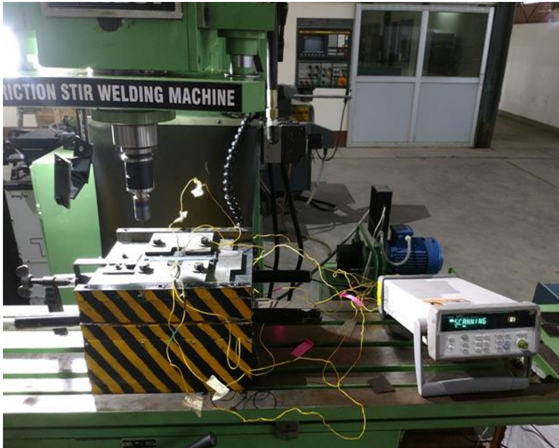
Figure 3.18: FSW machine with thermocouples and data acquisition system.
