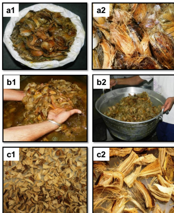
Figure 2.2: The pictorial images of (a1 and a2) collected raw husk, (b1 and b2) washing of raw husk, and (c1 and c2) cut raw husk after drying at 105°C.
