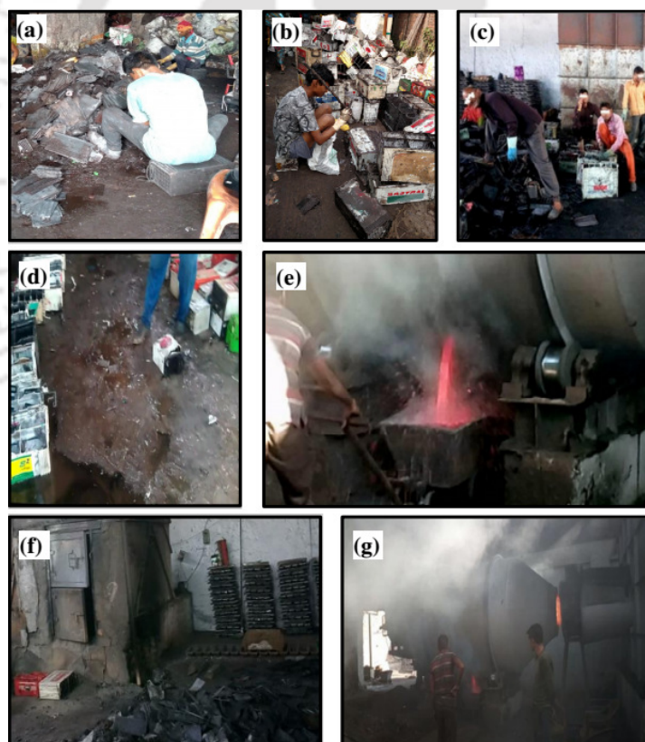
Figure 1.3: Crude, unhealthy, and illegal practices of ULAB recycling: (a) separation of lead grids, (b) and (c) breaking of batteries for lead recovery, (d) spillage of acid around in the battery, (e) lead fumes and spurt in trolley filing, (f) lead recovery furnace and (g) lead fumes during the rotary operation. (Pictures courtesy: (a) and (b) self-captured and (c), (d), (e), (f), and (g) are adopted from Trivedi (2017) [3]).
