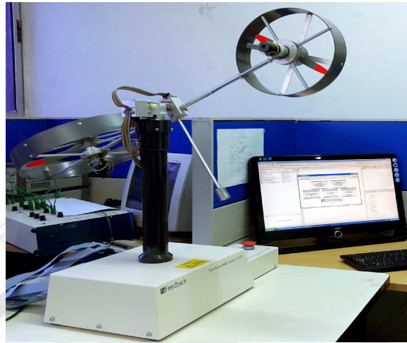
Figure 5.2: TRMS laboratory model
