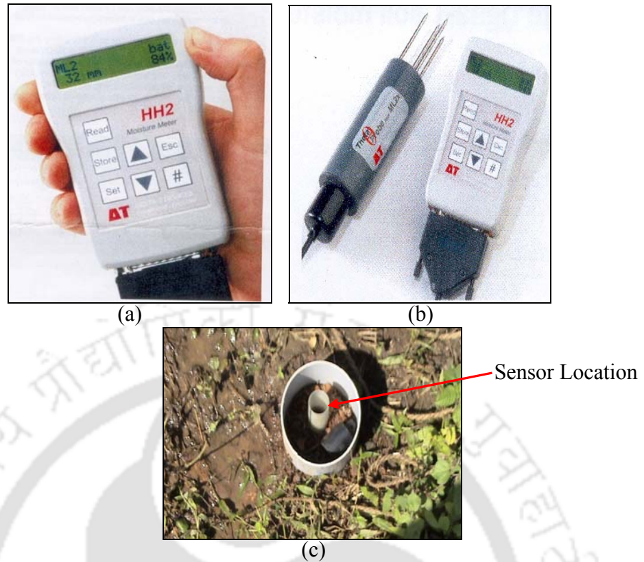
Fig. 3.22(a-c) Delta-T soil moisture meter (Type HH2)
