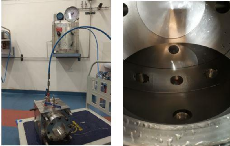
Figure A2-40 Hydraulic pressure test
