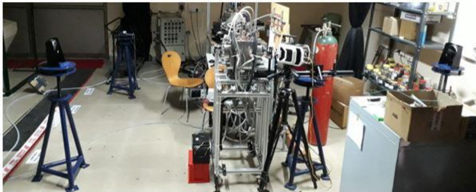
Figure A2-30 Schematic and Actual arrangement of shadowgraph system
