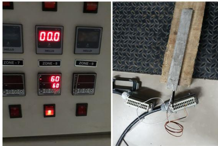
Figure A2-42 Temperature controller and heating cartridge test using a load cell
