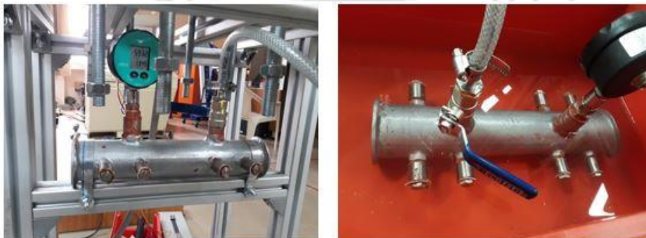
Figure A2-41 General leak and water immersion test for the pressure manifold
