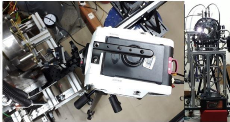
Figure A2-31 High-speed camera and light source of the imaging system
