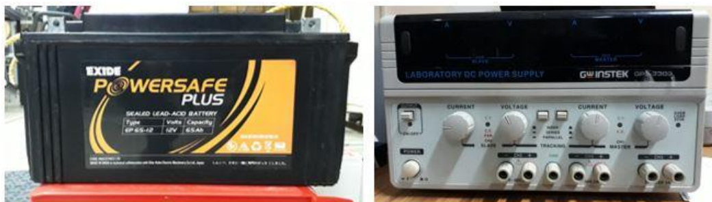
Figure A2-25 12V Acid Battery and Adjustable Digital DC power supply
