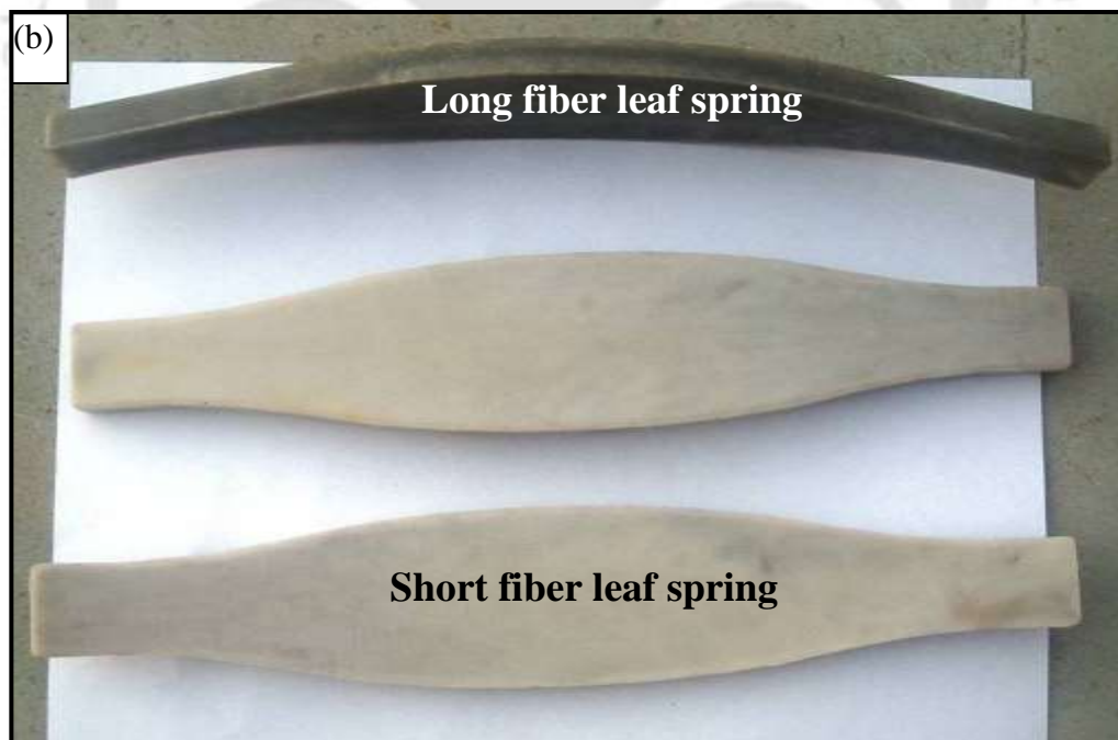
Fig.6.15b Photograph of the developed leaf springs
