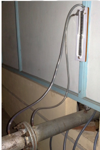
Fig.3.3 Orifice plate, D-D/2 pressure tapings connected with manometer board
