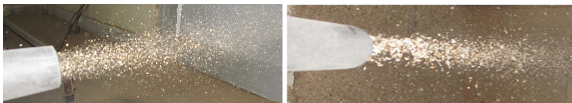
Fig.7.30 Flow of biomass for the particle size of 732\ \mu\text{m} at low speed
