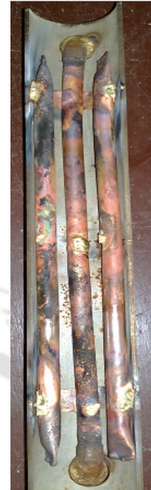
Fig.3.11 Heat transfer probe-2 (without twisted tape)
