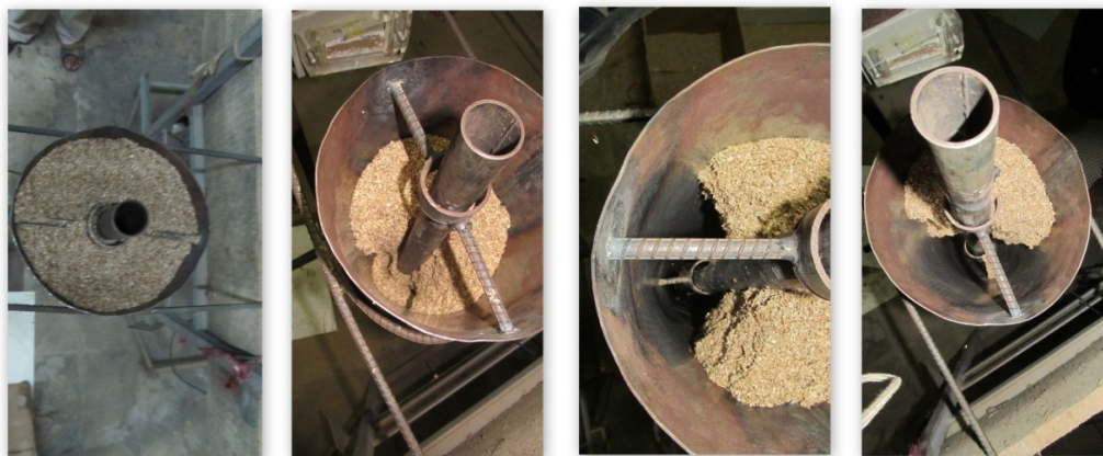
Fig.7.28 Snapshot of the inside of the cone feeder in intervals of 30 seconds
