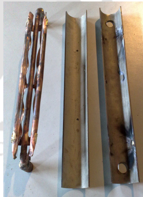
Fig.3.12 Heat transfer probe-3 (with twisted tape)
