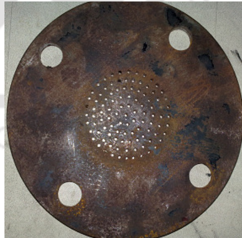
Fig.3.4 Straight hole type distributor plate
