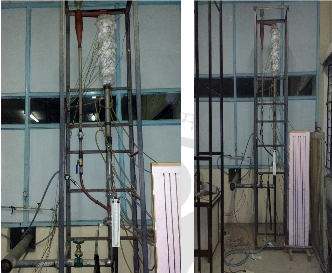
Fig.3.2 Photograph of the cold PCFB experimental setup
