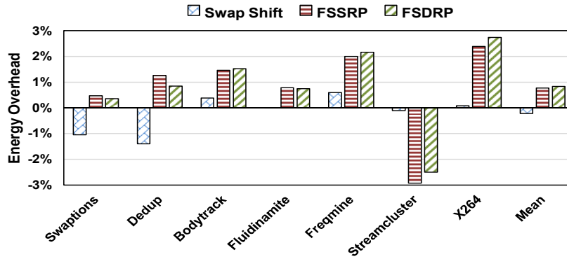
FIGURE 6.9: Energy overhead by the proposed techniques: FSSRP and FSDRP against baseline STT-RAM (lower is better)
