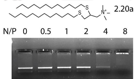
Figure 2.43. Electrophoretic gel retardation assay of pMMP7-GFP in the absence and presence of co-liposomes at different N/P ratios (0 to 8). The molar ratio of synthetic lipid ( 2.20a ) and PE was 1:1.
