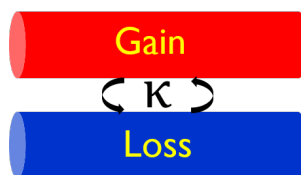
Figure 2.1: Schematic of a \mathcal{PT} -symmetric directional coupler. The coupling co-efficient is denoted by \kappa .
