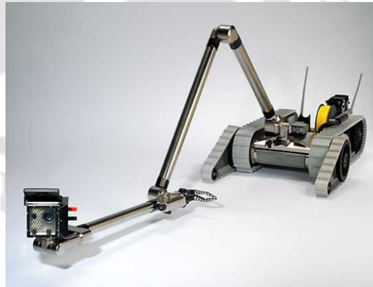
Fig. 1.4. Multi-role flexible robot for hazmat handling, search and rescue, and hostage rescue operation. ( www.armedforces-int.com/ )
