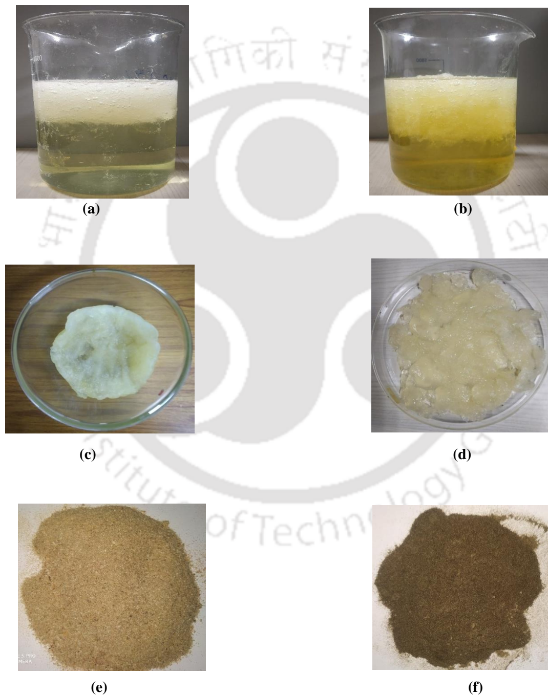
Fig. 6.10: Macrographs of precipitated pectin (a and b), wet pectin (c and d) and dried blended pectin (e and f) obtained by pulsed UAE and acidic hot water extraction process respectively.
