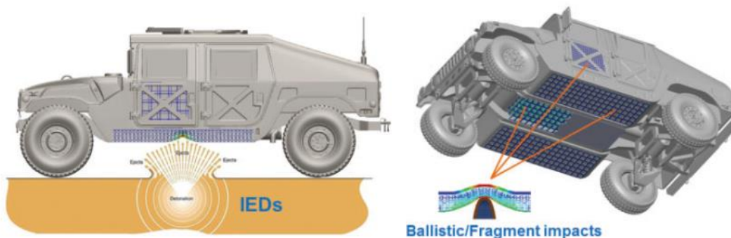
Figure 2.12. Applications of auxetic structures to improve the impact resistance of armored vehicles (Reproduced with permission from [57]).
