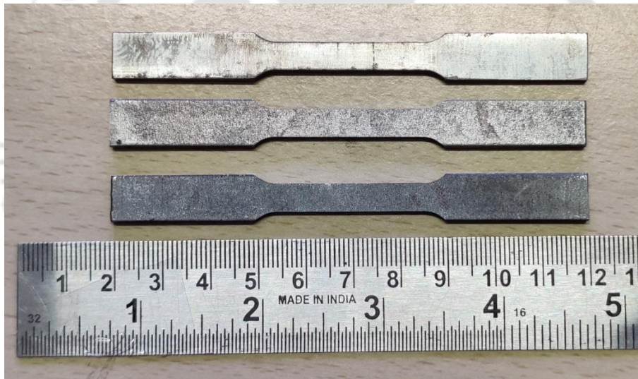
Figure 3.2. ASTM E8 AlSi10Mg tensile specimens fabricated by Selective Laser Melting.
