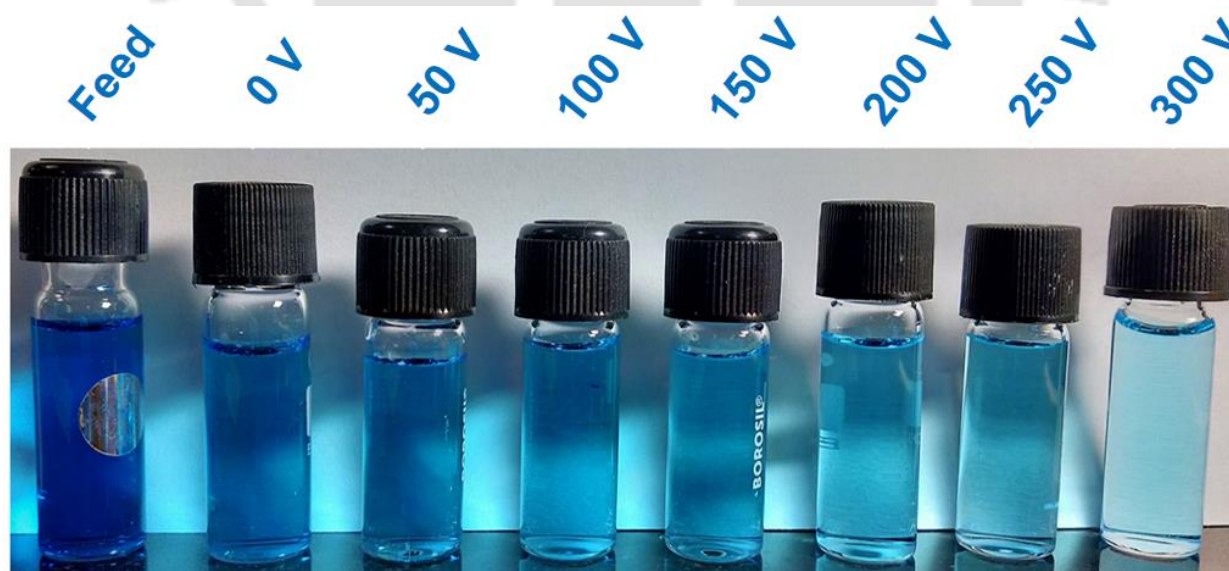
Figure 4.6 Shows the images of glass vials containing aqueous phase samples of feed, 0 V, 50 V, 100 V, 150 V, 200 V, 250 V, and 300 V for highest (E5) number of electrodes.
