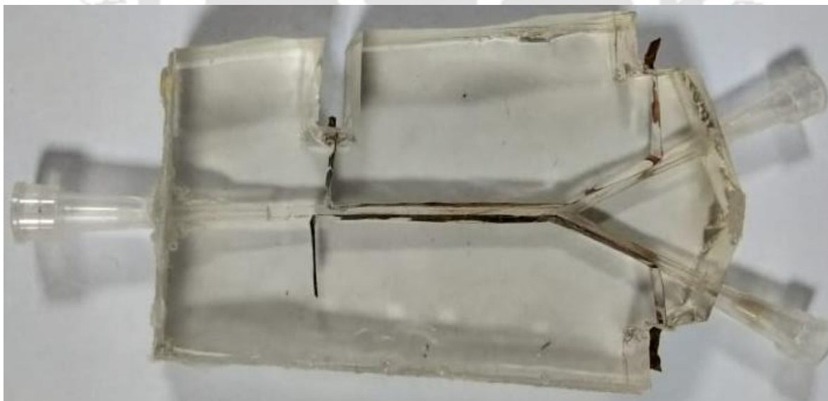
Figure 3.1 Shows the optical image of Y-shaped electrode embedded microchannel.
