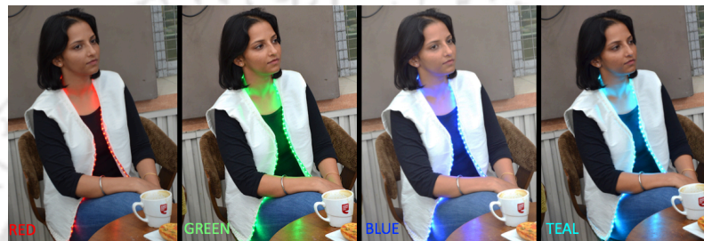
Figure 4.32: Model wearing dynamic jacket – colors being controlled by a wireless remote
