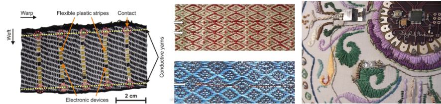
Figure 2.24: Woven smart fabric; Figure 2.25: Woven sensors, University of Laval; Figure 2.26: LilyPad Arduino embroidered on fabric
