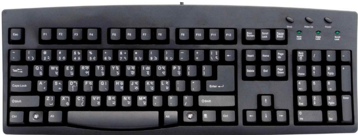
Figure 2.15: In-script Assamese/Bengali physical keyboard for computer typing developed by Bijoy
