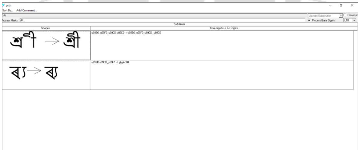
Figure 6.33: Configuration of the combination of core and upper modifier characters in MS Volt
