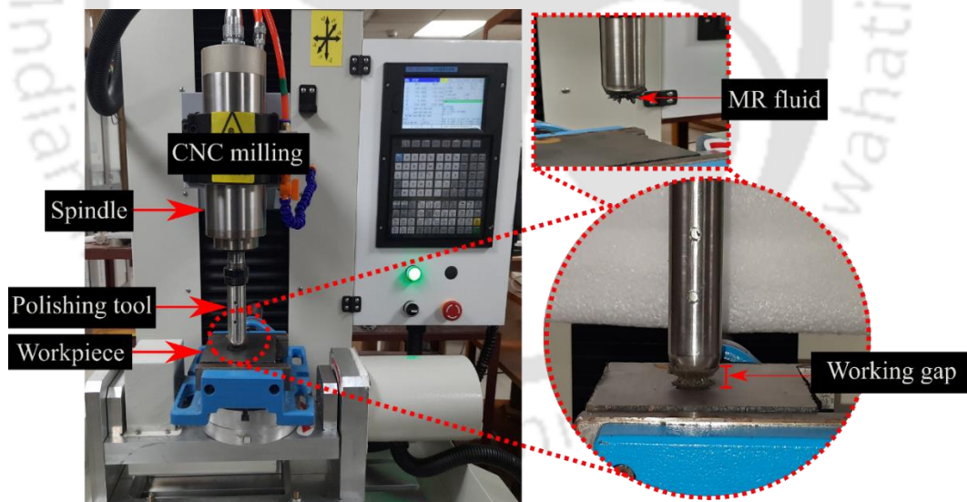
Fig. 2.3 Experimental setup of magnetorheological finishing
