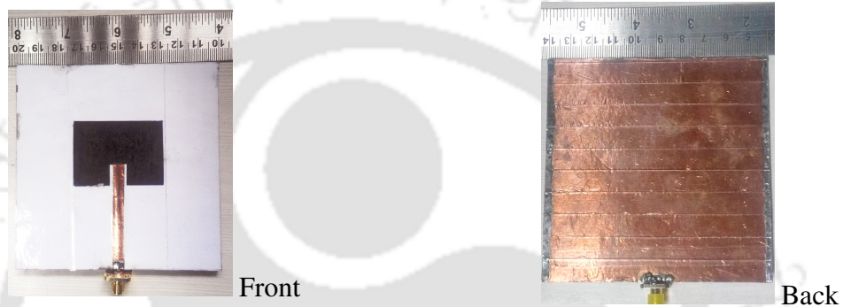
Figure C.1: Microstrip antenna fabricated using GNP based ink and an atomizer.
