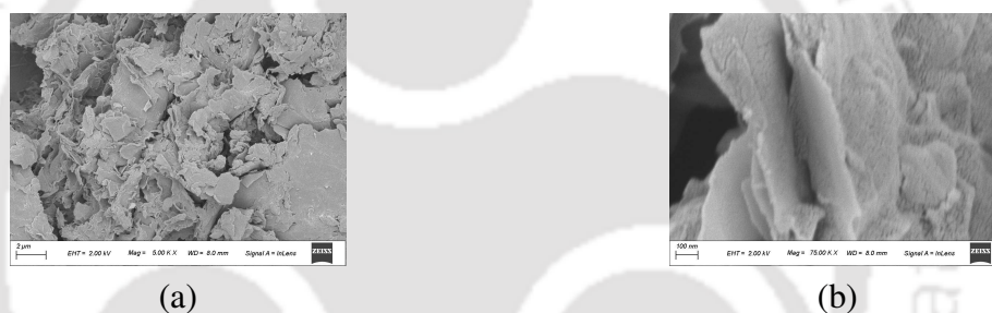
Figure 5.31: FE-SEM images of FLG sample from Graphite plate obtained at CIF, IIT Guwahati
