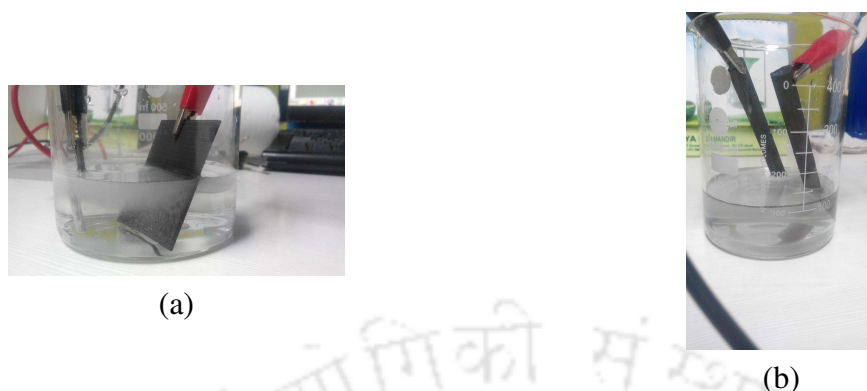
Figure 5.28: Electrochemical Exfoliation of Graphite in our Laboratory, at IIT Guwahati (a) Plate form (b) HOPG rod
