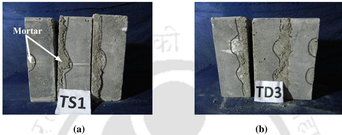
Figure 5.9 Failure behavior of AAC masonry triplet: (a) debonding of middle block-mortar interface and (b) debonding of side block-mortar interface
