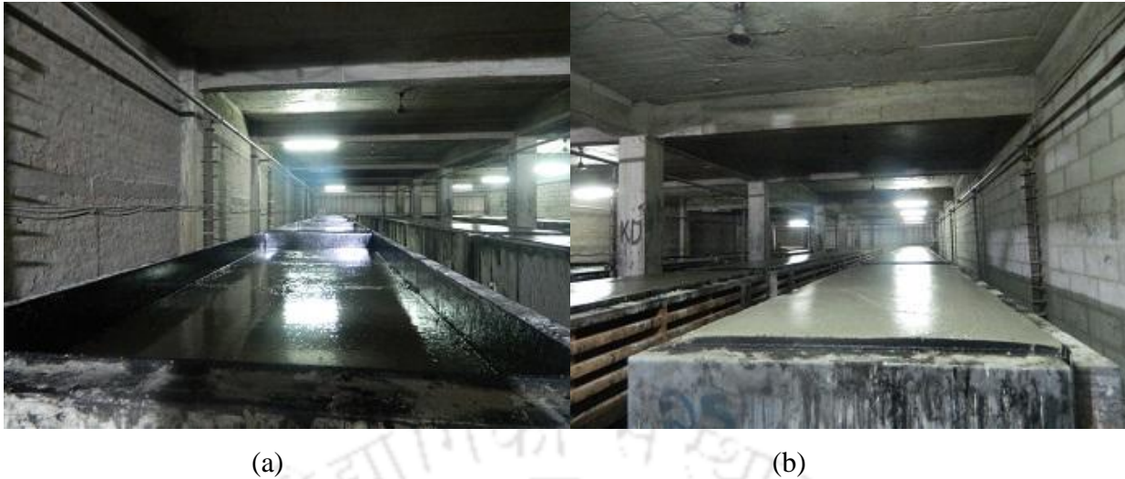
Figure 1.5 Photographs of mold (a) mold partially filled with slurry just after pouring and (b) mold fully filled with slurry after the expansion or pre-curing process
