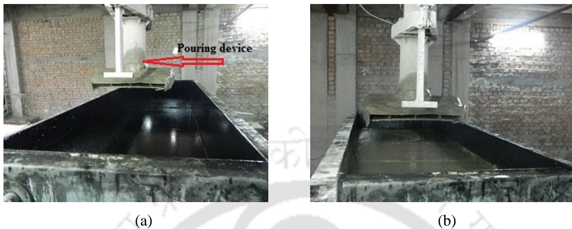
Figure 1.4 Photographs of mold and pouring device (a) position of mold and pouring device and (b) pouring of the slurry into the mold
