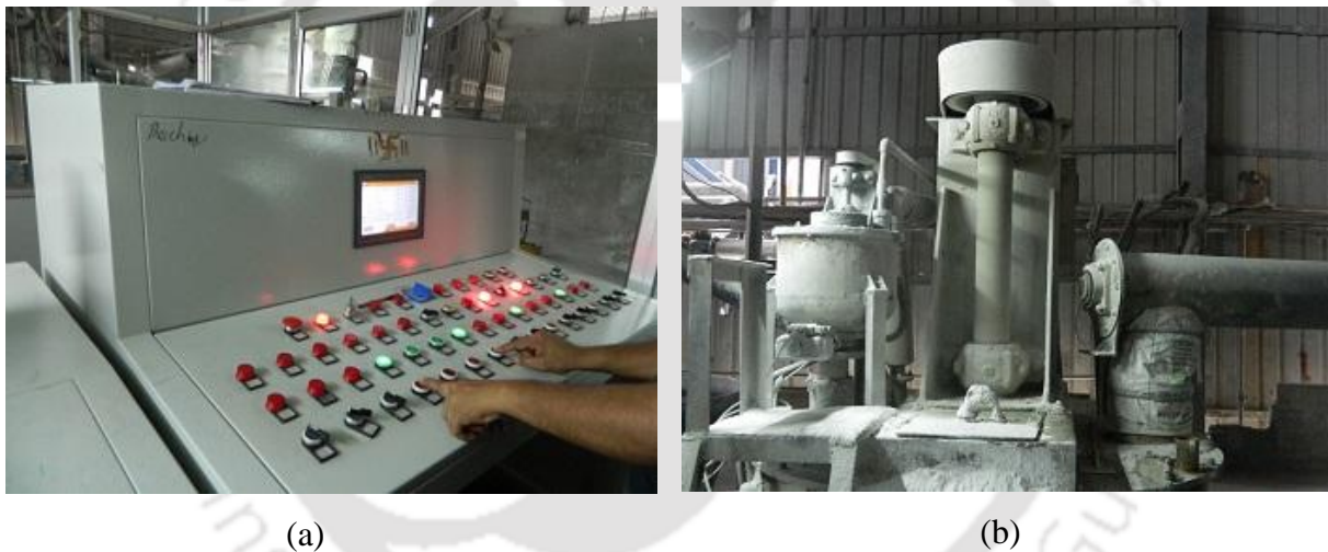
Figure 1.3 Photographs of devices used for mixing process (a) PLC automatic system to control mix proportions and (b) machine for mixing raw materials
