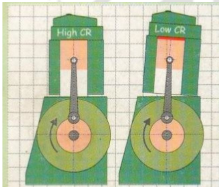
Figure 3.4: Principle of tilting cylinder block assembly.
