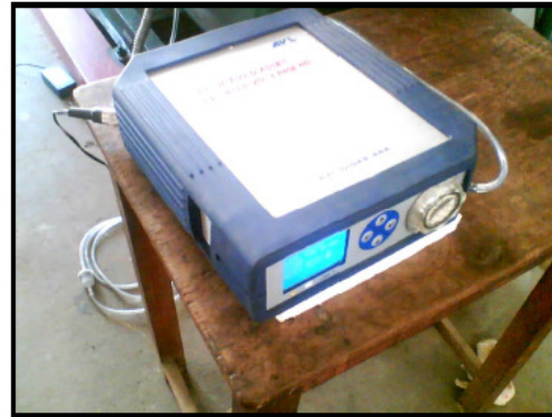
Figure 3.9: Photographic view of the exhaust gas analyser.
