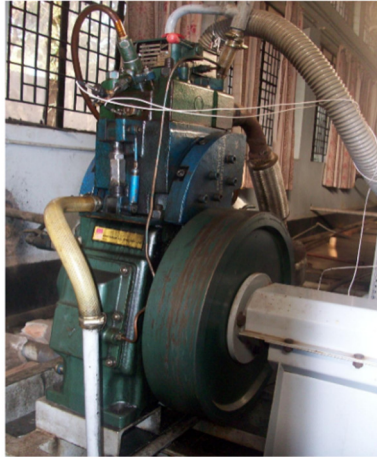
Figure 3.2: Variable compression ratio diesel engine.
