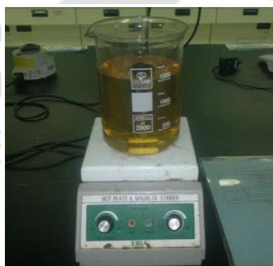
Figure 4.2: Fuel preparation using magnetic stirrer.
