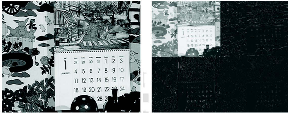
(a) Original image of Frame 1 of Mobile(CIF) Sequence (b) Decomposed image into four subbands
