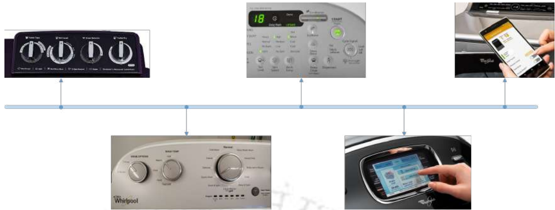
Figure 2. 3 A rough visualization showing evolution of a household washing machine user interface Source: Whirlpool Corporation
