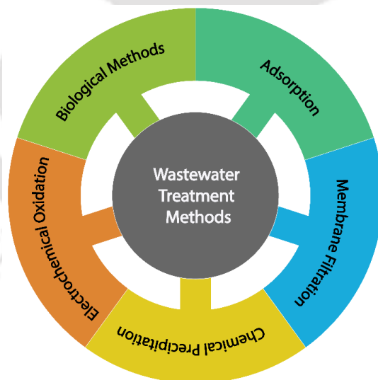
Figure 1.2. Schematic diagram illustrating commonly used water treatment methods, encompassing physical, chemical, and biological approaches to effectively remove contaminants and improve water quality in various wastewater treatment plants.
