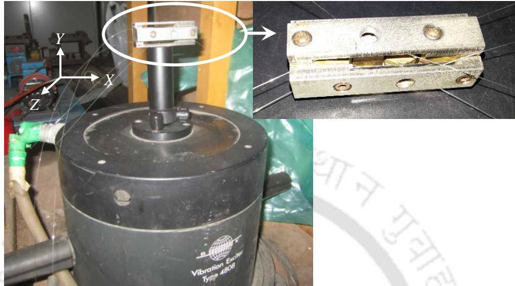
Figure 4.4: Experimental set-up for the characterization of proposed optical fiber vibration sensor. Inset shows the proposed sensor.
