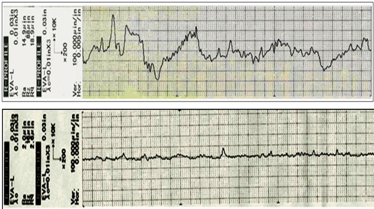
Fig. 4. 11 (a) Surface of the test material before testing; (b) Surface of the test material after testing: straight WC-Co. (c) Surface of the test material after testing: WC-Co-5wt. % CaF 2 .
