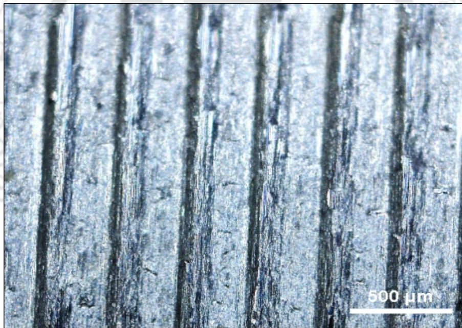
Fig 5.13(a) Surface of the workpiece machined by developed material (WC-Co-5 wt.% CaF 2 ) under velocity of 80 m/min
