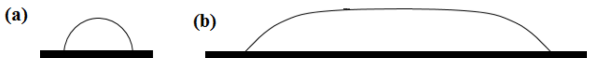
Figure 1.1. The shape of the liquid droplet by placing the droplet on a horizontal surface:
