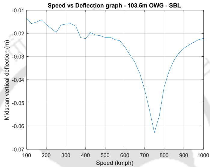
Fig. 5.5. Midspan vertical deflection at different speed for 103.5 m span OWG with SBL
