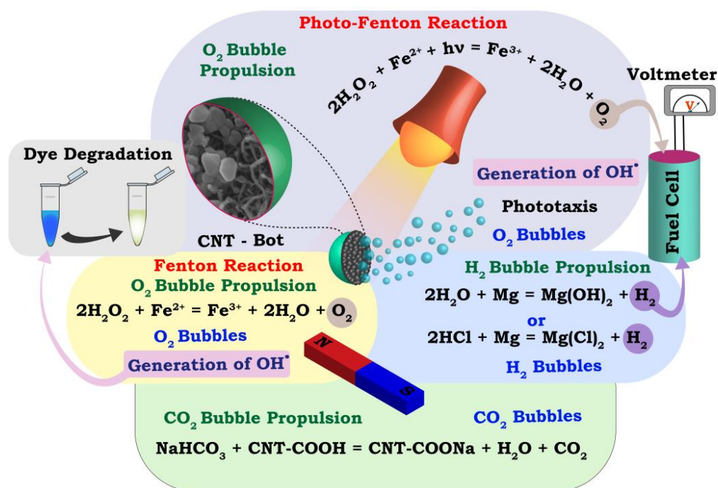
Figure 5.1: Schematically shows a CNT-bot composed of a –COOH functionalized MWCNT cluster doped with a ferrous ( \text{Fe}^{2+} ) salt and magnetite nanoparticle ( \text{FeONPs} ) before coated with a Mg film. The CNT-bot was capable of undergoing two reactions in acidic and alkaline water (e.g. \text{Mg} + \text{H}_2\text{O} \rightarrow \text{Mg(OH)}_2 + \text{H}_2 , \text{Mg} + \text{HCl} \rightarrow \text{Mg(Cl)}_2 + \text{H}_2 and \text{NaHCO}_3 + \text{MWCNT-COOH} \rightarrow \text{MWCNT-COONa} + \text{H}_2\text{O} + \text{CO}_2 ) and Fenton reaction (in absence of light) and Photo Fenton reaction (in presence of UV light) in the peroxide fuel ( \text{Fe}^{+2} + \text{H}_2\text{O}_2 \rightarrow \text{Fe}^{+3} + \text{H}_2\text{O} + \text{O}_2 ), as shown on the image. Subsequently, the motor moved by the ejection of hydrogen bubbles in acidic water, carbon-dioxide propulsion in the alkaline water, and oxygen bubbles in the peroxide fuel. The motors could show directionality in the motion under acid and alkali gradients leading to acid- and alkali-taxes, as shown on the images. The scheme also shows that hydrogen and oxygen serve as fuels of PEM Fuel cell and the CNT-bot can also perform dye degradation function.
