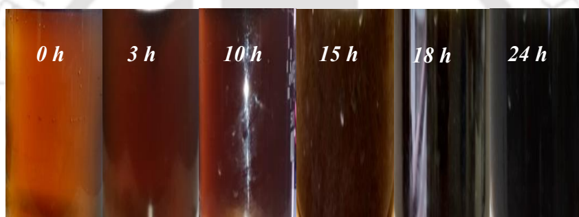
Figure 4.7. Variation of PtCoNPs(1:1) color intensity with synthesis time.
