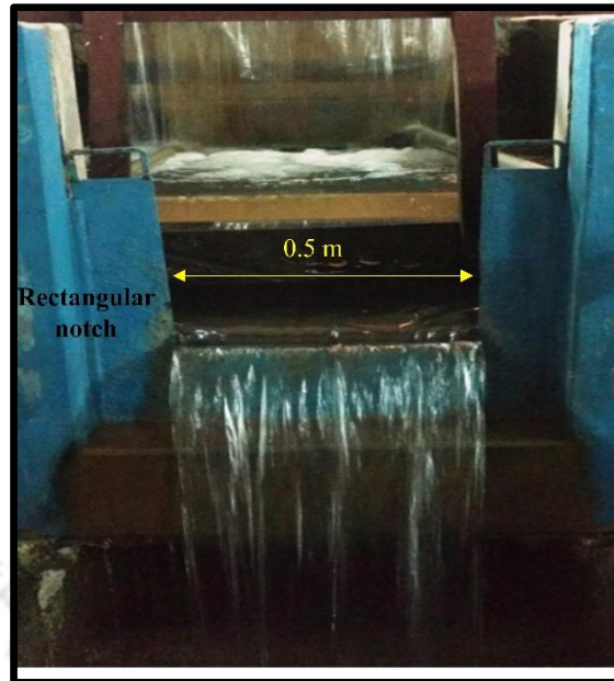
Figure 2.5 Discharge measurement at rectangular notch
