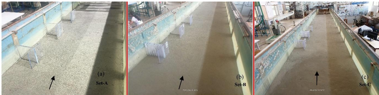
Figure 2.18 Experimental bed conditions before run with different sets of permeable spur dikes, Set-A (a), Set-B (b), and Set-C (c).
