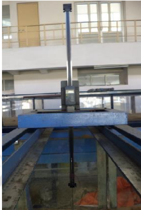
Figure 2.7 Digital point gauge mounted on moving trolley
