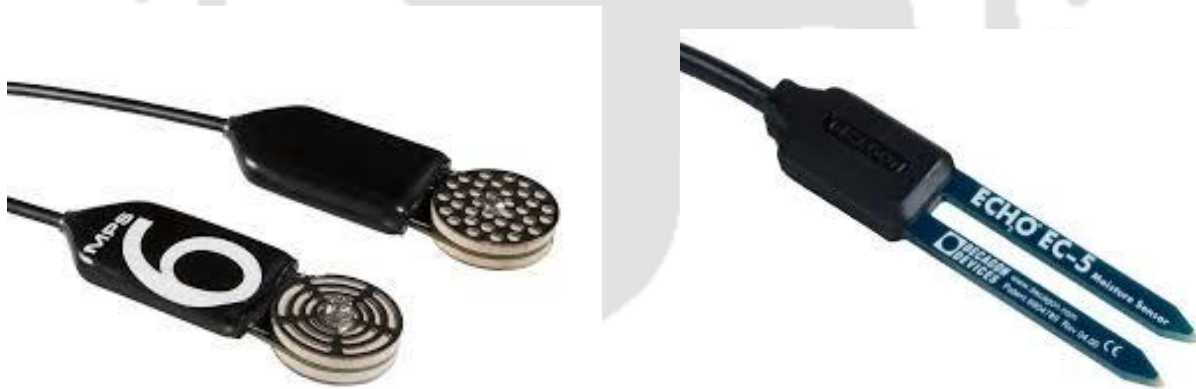
MPS6 sensor for suction measurement
