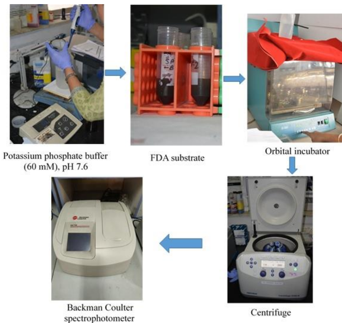
Fig.3.12 Microbial activity determination stages by FDA analysis
