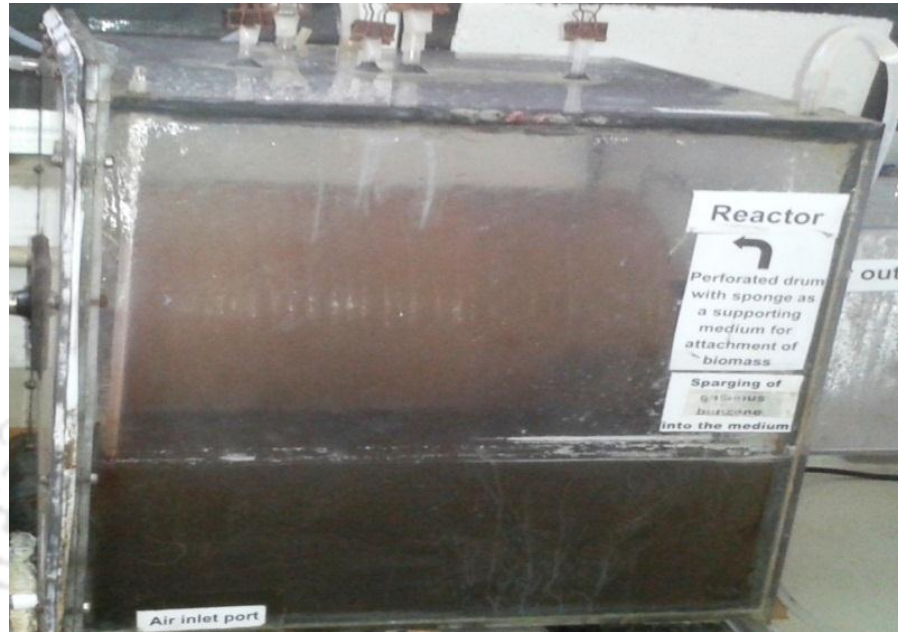
Fig. 5.1 Biofilm developed on RBC at 30 th day
