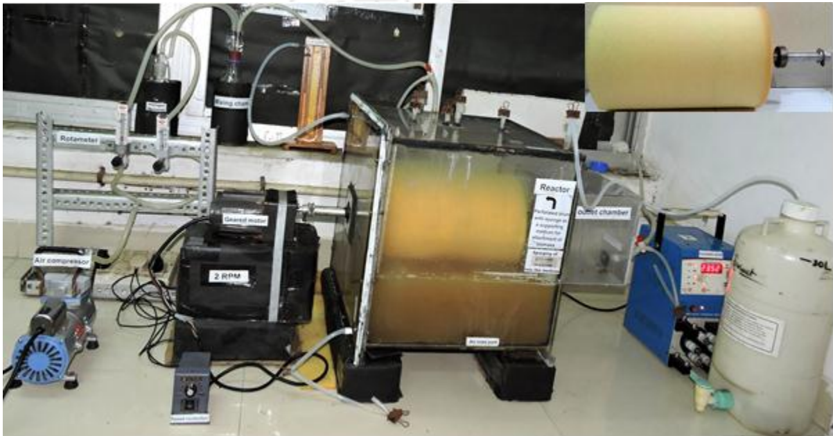
Fig. 3.2 The RBC after design and complete installation in picture
