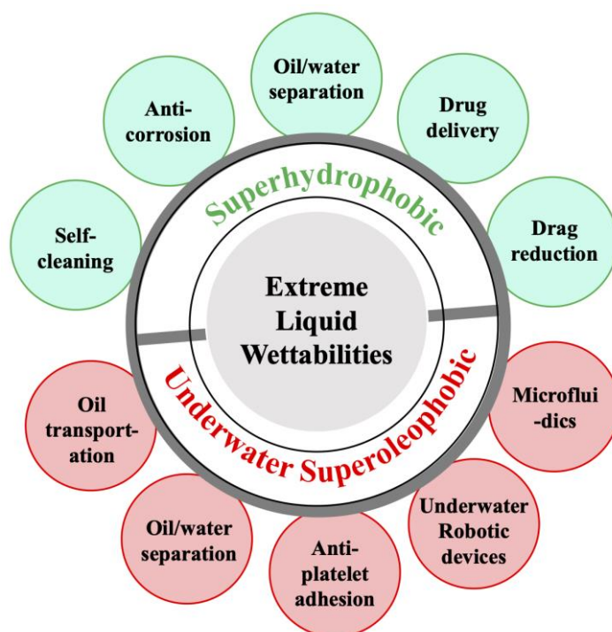
Figure 1.18: Accounting various applications of both superhydrophobic (in air) and superoleophobic (under water) properties.
