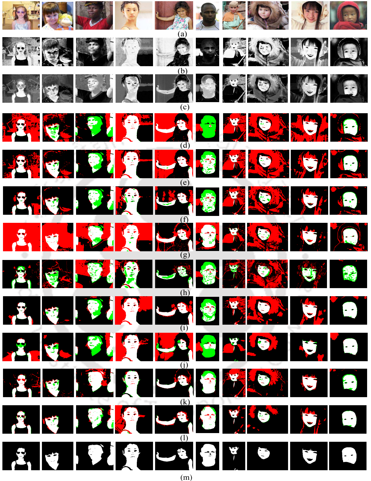
Figure 3.10: Skin segmentation results : a) Original image, b) SPM, c) Proposed FSPM, d) SPM + direct threshold [13], e) DSMSC [19] + direct threshold, f) DSMSC [19] + FPSS [14], g) DTSC [20], h) SHSC [10], i) ASSC [21], j) DSPF [9], k) FSPM_{Face} + direct threshold, l) FSPM_{Face} + DRG, and m) Ground truth. Here, white colour represents true positive , black colour represents true negative , red colour represents false positive , and green colour represents false negative .
