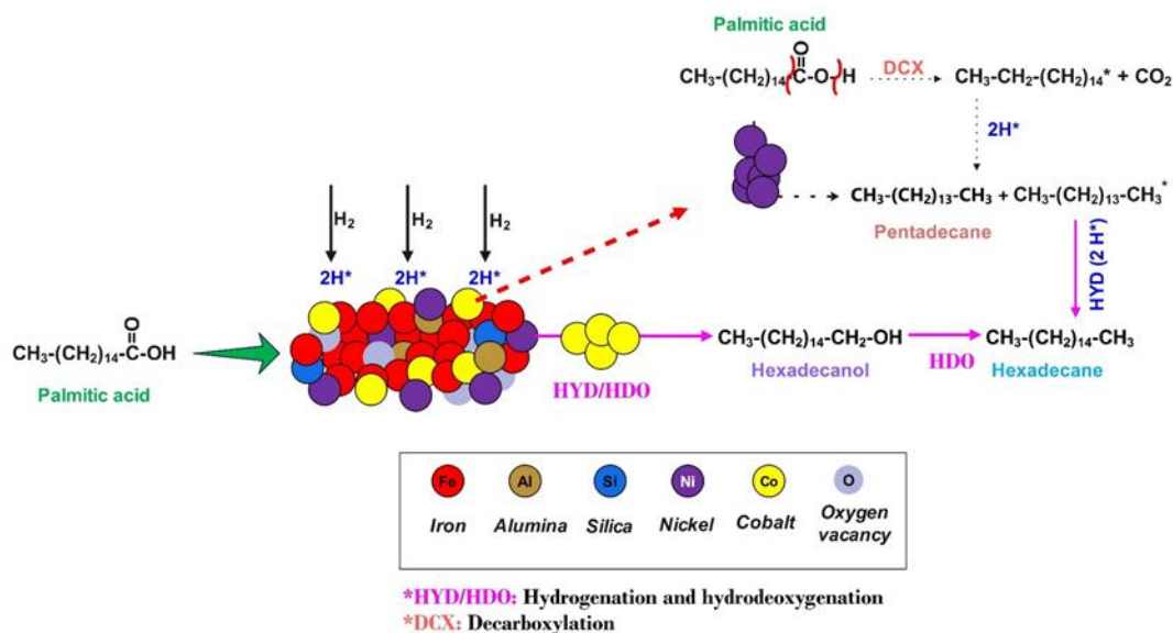
Figure 33. Reaction mechanism describing the conversion of palmitic acid
