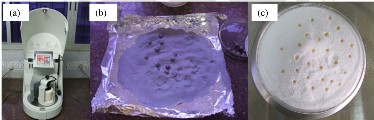
Figure 3.3 a) Ball milling machine b) MWCNTs blended UHMWPE c) \alpha_T lumps in UHMWPE prior to ball milling
